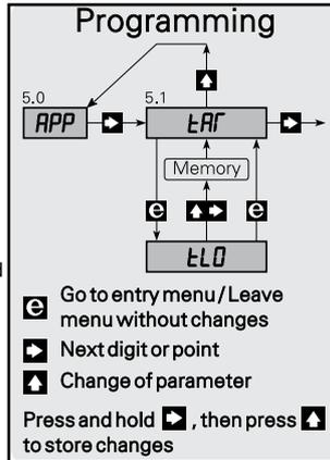
When submenu 5.1 has been selected for {tLO or tHI}, activating the  $\left[ \left[ \left[ \right] \right] \right]$  key for more than 2 s will tare the input value to the value it had when activated. The input span is not affected but is kept relative to the new offset value.
